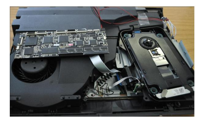
You can now attach the plastic clips to the clip on PCB as per drawing below and secure to the back of your console as shown here (CECH25XX/3XXX) (Refer to table at the beginning of guide for usage/allocation of clips):
