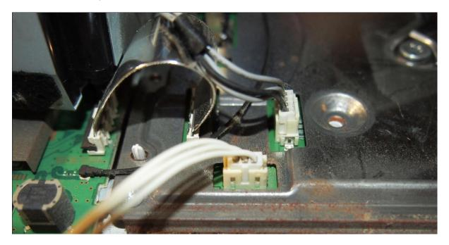
Replace the cable with the correct type which has the connector matching that of your console. Kindly, note carefully the orientation and direction of the cable, failure to do so could cause damage or malfunction.
