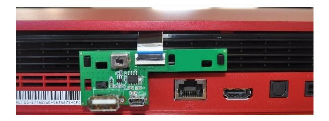
You can now attach the plastic clips to the clip on PCB as per drawing below and secure to the back of your console as shown here (CECH4XXX) (Refer to table at the beginning of guide for usage/allocation of clips):
