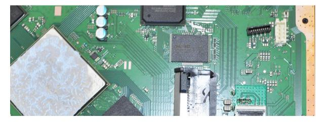
Should you wish to restore you motherboard to it original state, carefully de-solder de QSB then cleanup the solder traces and re-solder the original capacitors or replacement capacitors (10nf)
