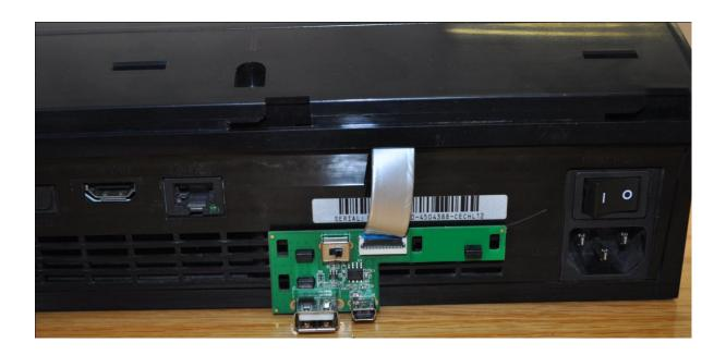
You can now attach the plastic clips to the clip on PCB as per drawing below and secure to the back of your console as shown here (CECH 2XXX/21XX) (Refer to table at the beginning of guide for usage/allocation of clips):
